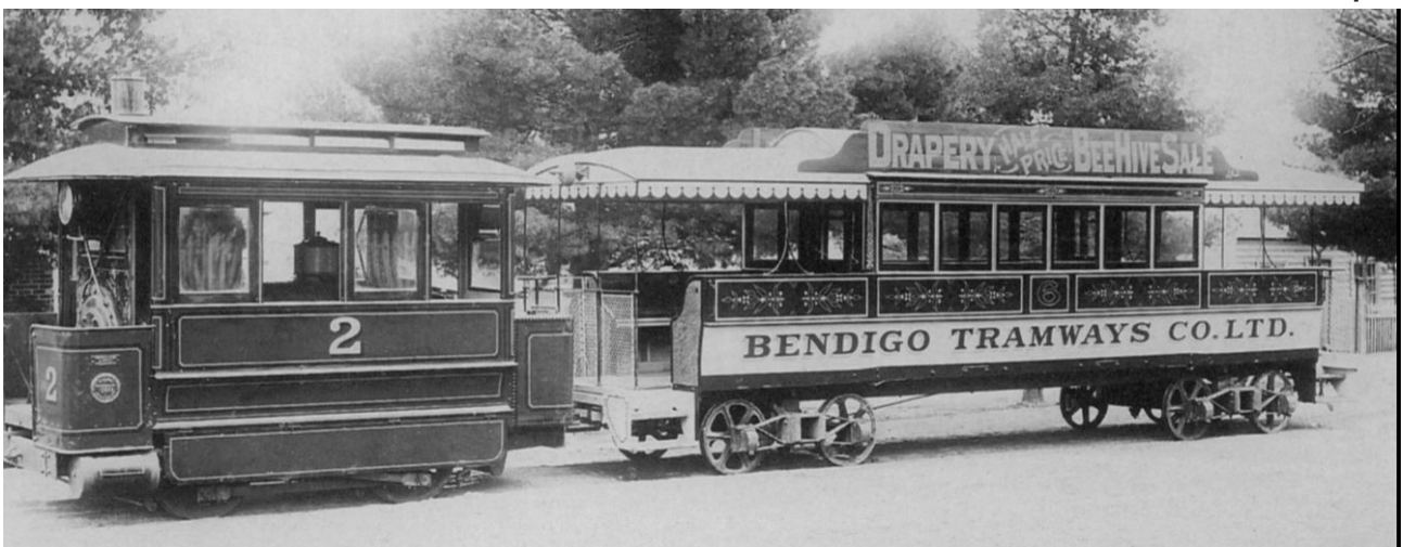
Bendigo Tram engine No.2 and bogie trailer No.6, c.1892. The engine was one of two from Bendigo that David Mitchell purchased for the Cave Hill tramway in 1903. The engine was dark red and gold with a green boiler, the bogie red and cream with gold and blue lettering . Photo courtesy Bendigo Tramways.
