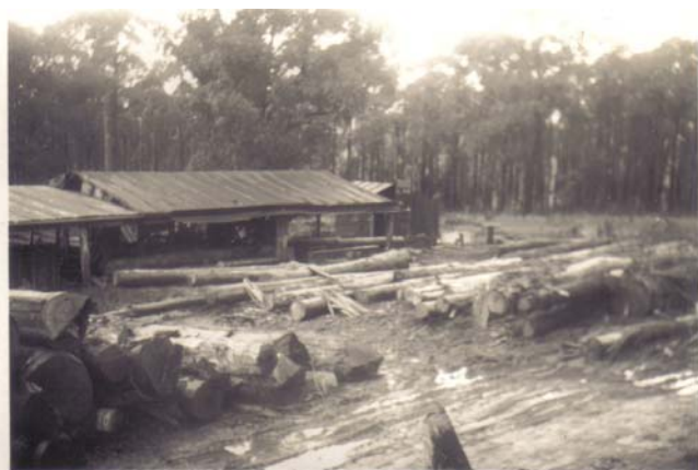
Above left, machinery shed and timber yard with unsawn logs. Above right, logs and machinery. Note the two axes in one log. It appears the logs were trimmed with axes before being sawn.
